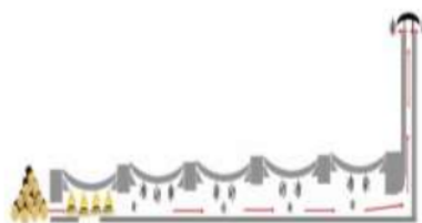
Sketch of energy-efficient cooking stove
